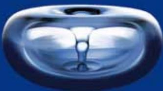
Multiply enlarged cavitation bubble in the moment of implosion
